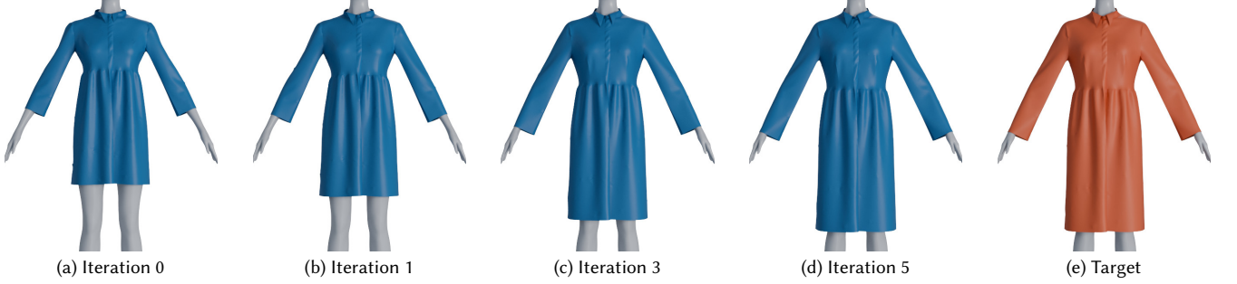
Fig. 12. Cloth rest-scale fitting on a fixed mannequin. The blue panels show the initial drape and results after 1, 3, and 5 updates. The orange panel shows the target.
