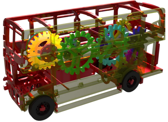
Fig. 24. Diagonal view of the London bus. The yellow gear acts as the motor, driving the bus forward through rolling friction between the wheels and the ground. The wheels are simulated as rubber using FEM, while all other parts are modeled as stiff affine bodies. Detailed simulation setup is provided in Table 4.
